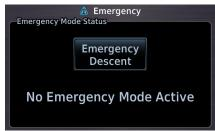
If configured for cabin pressure monitoring, the system monitors cabin pressure once EDM is armed. EDM is considered armed when:
