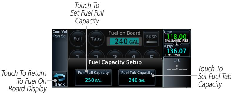
Figure 1-14 Fuel Capacity Setup Page
