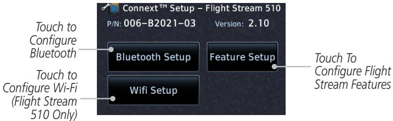
**Figure 15-51 Connex Setup for Flight Stream 510**
