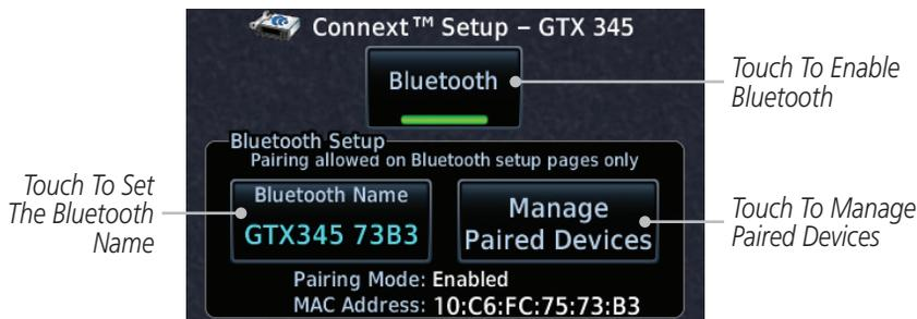
**Figure 15-57 Connex Setup for GTX 345**
