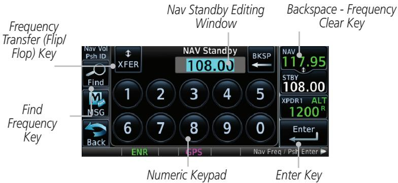
**Figure 3-6 Nav Standby Frequency Numeric Keypad**
