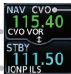
Nav Frequencies Will Automatically Decode Morse Code And Display The Ident
