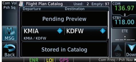
**Figure 4-66 Catalog for Multiple Flight Plan Import**
