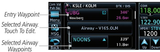
Figure 4-24 Airway Waypoints in the Flight Plan
