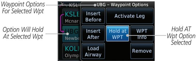
Figure 4-26 Active Flight Plan with Hold At Waypoint Option
