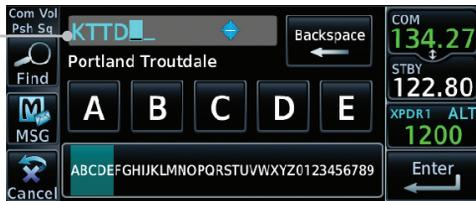
Figure 4-12 Use the Alphanumeric Keypad to Select Waypoint to Insert Before
