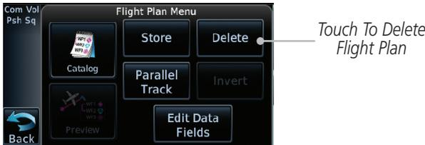
Figure 4-3 Delete Existing Flight Plan
