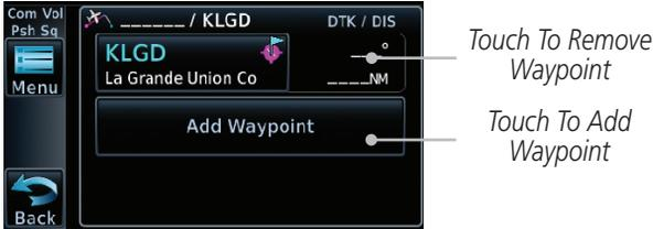
Figure 4-2 Create New Flight Plan
