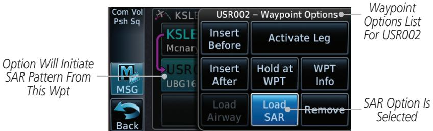
Figure 4-28 Active Flight Plan with Load SAR Option
