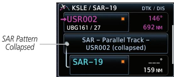
Figure 4-31 SAR Pattern Collapsed in Flight Plan
