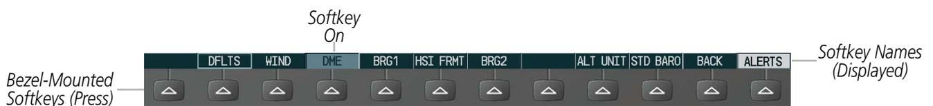
Figure 1-14 Softkeys (Second-Level PFD Configuration)
