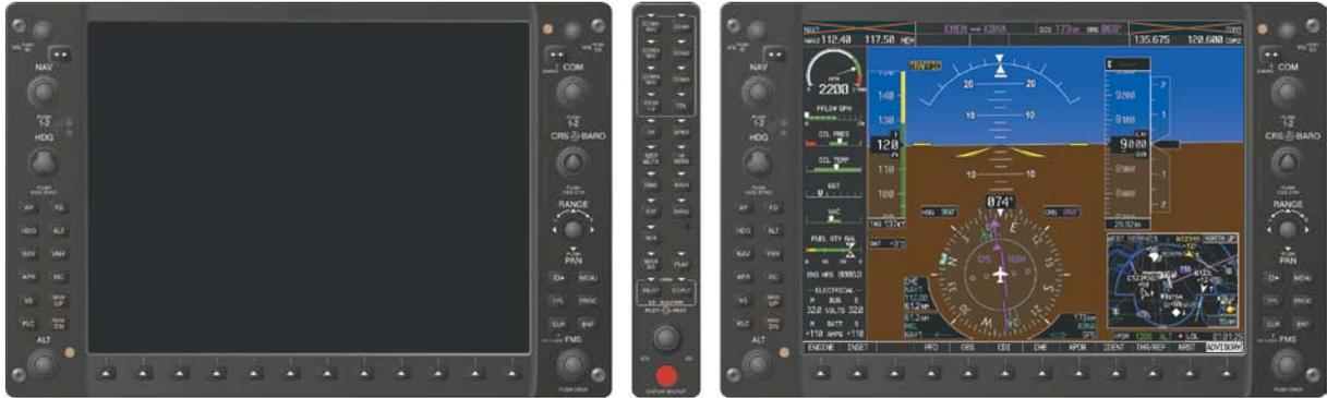
Figure 1-10 Reversionary Mode (Failed PFD)
