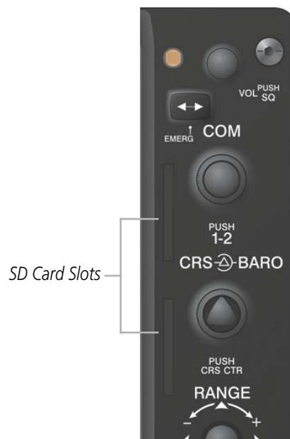
Figure 1-6 Display Bezel SD Card Slots
