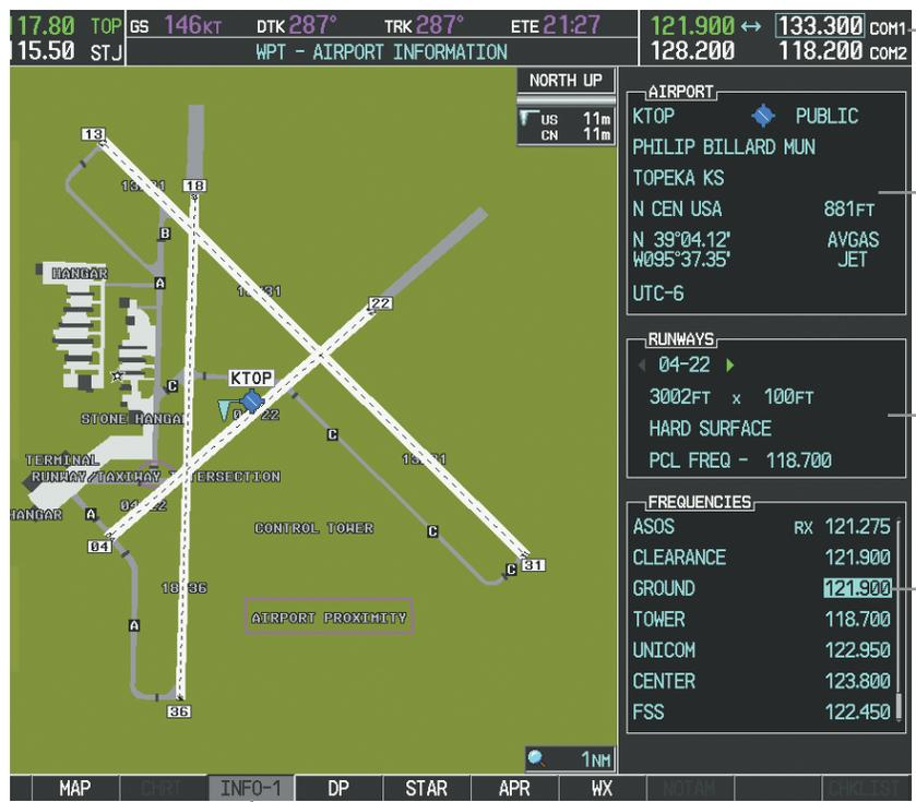
Press **Frequency Transfer** Key to Load Frequency into COM Active Frequency Field
