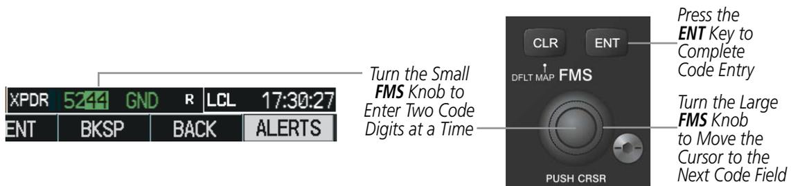
Figure 4-37 Entering a Code with the FMS Knob
