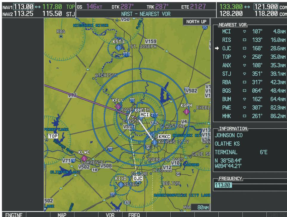
Press the **ENT** Key to Load the Frequency into the NAV Standby Field.
