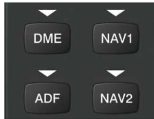
Figure 4-18 Selecting a NAV Radio Receiver
