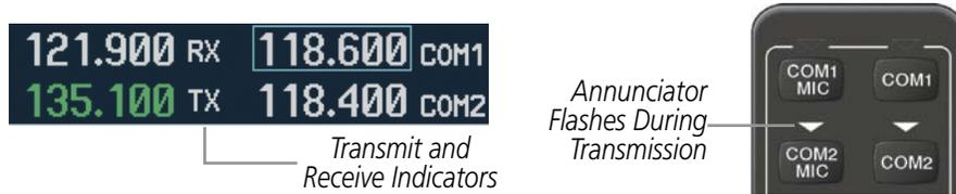
Figure 4-4 COM Radio Transmit and Receive Indications
