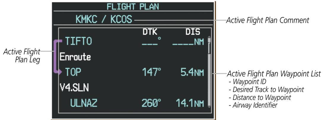
Figure 5-57 Active Flight Plan Window on PFD
