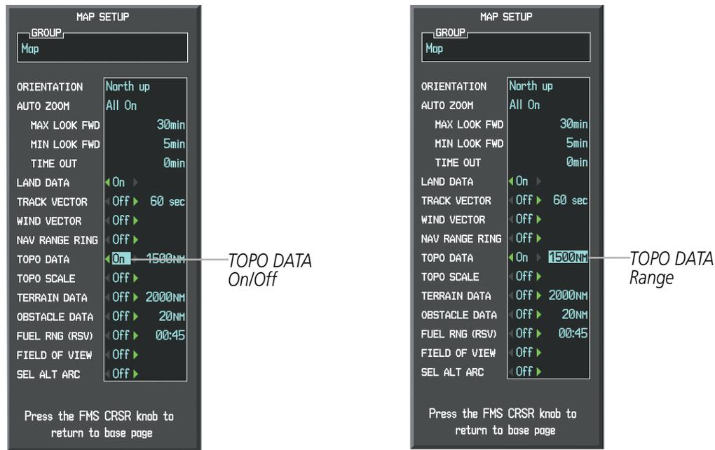
Figure 5-15 Navigation Map Setup Menu - TOPO DATA Setup
