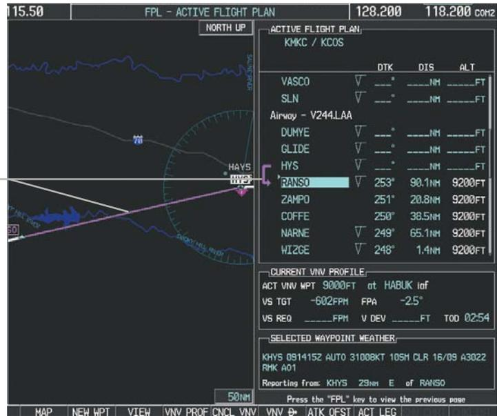
Figure 5-85 Active Flight Plan Page - New Active Leg
