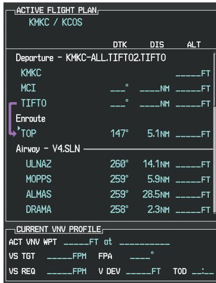
Figure 5-66 Active Flight Plan Page - Airway Inserted
