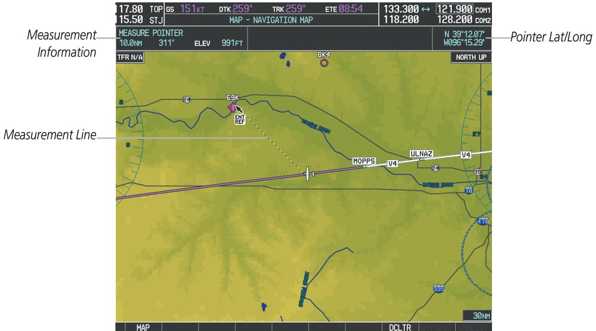
Figure 5-13 Navigation Map - Measuring Bearing and Distance
