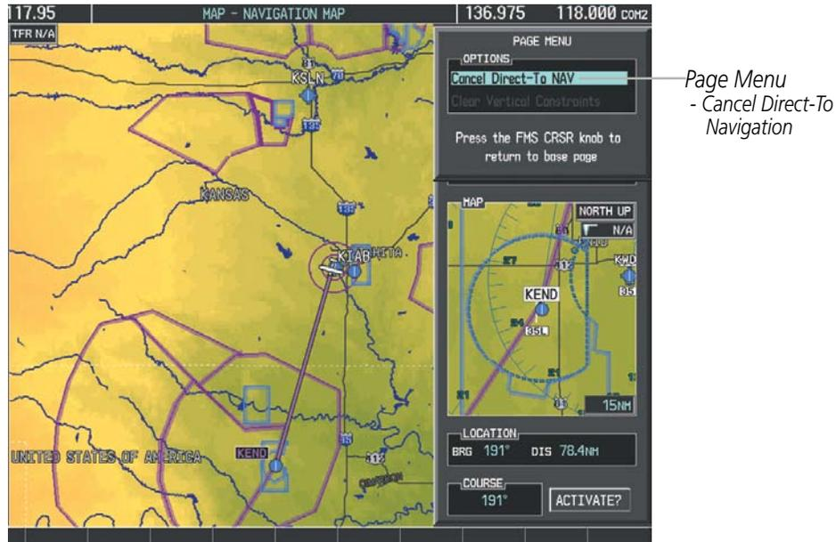
Figure 5-54 Direct-to Window - Cancelling Direct-to Navigation
