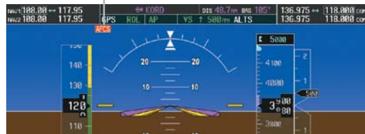
Figure A-6 AFCS System Status Field
